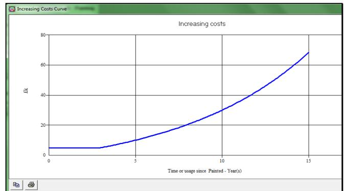
Figure 3. Escalation of painting cost with preparation needs
